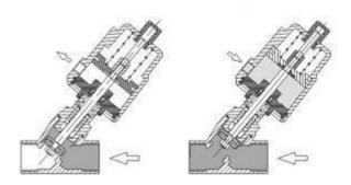
Simple Effect Actuator (Spring Return) Normal Closed (N.C.)
