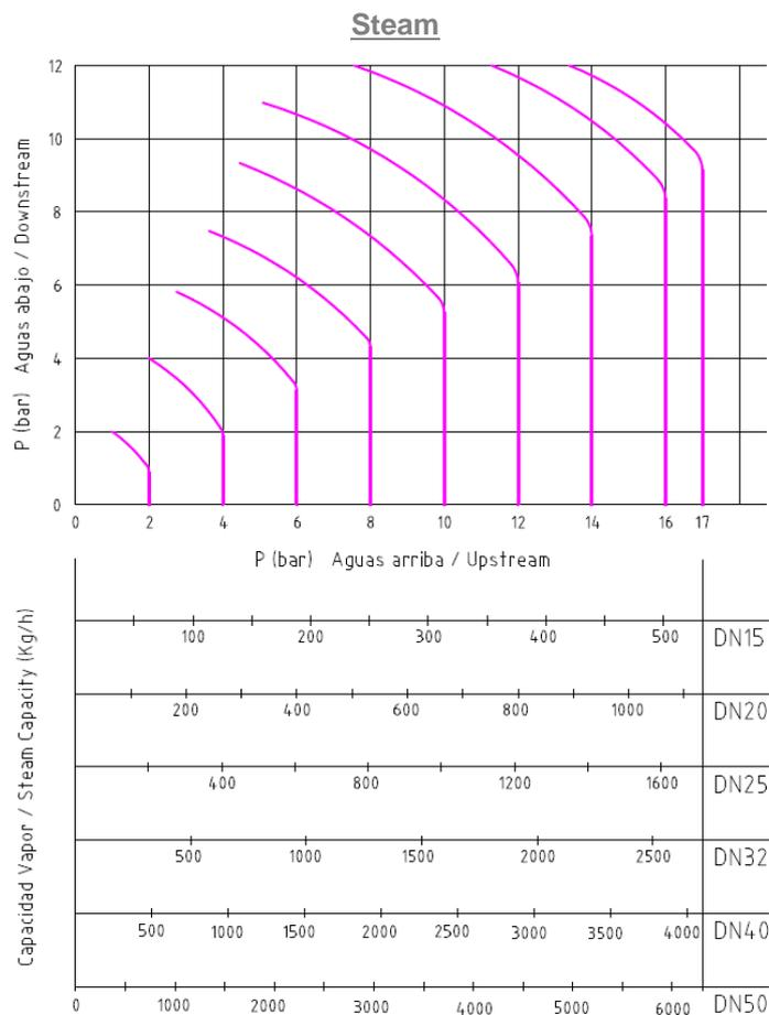
**Example:** a valve size DN40 reducing from 10 bar (upstream) to 7 bar (downstream) is able to flow until 2000 Kg/h of steam, approximately.
