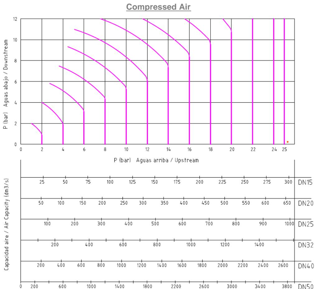
The previous diagrams show the discharge capacity of the pressure reducing valves of GENE BRE, S.A. art. 2274 / 2274N / 2275, according to the relationship between the Inlet Pressure (P1) and the Outlet Pressure (P2), for both steam and compressed air.
