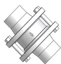
**ATTENTION:** in case you need to install the without spring, it can only be placed in vertical position (ascendant fluid).
